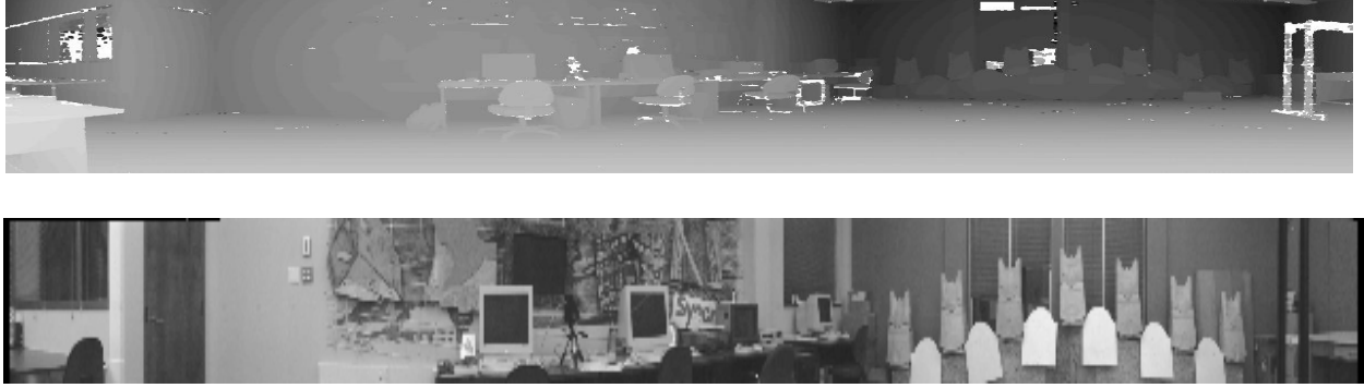
Figure 3: Spherical representation of the range data from an 180° scan after filtering (top). Corresponding 180° panoramic image mosaic (bottom).
