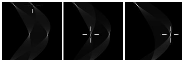
Figure 2: Identify and Remove cluster detection algorithm. 3 iterations (left-to-right) on the image in 1. The peak around the maximum value in the PH transform image is identified and the contributing pixels are identified by linked list E (see Fig. 3). The effect of these pixels is removed from the hough image for the next iteration.
