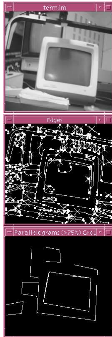
Figure 14: Top image: the original image; middle image: The edge detection and segments classification result; bottom image: the parallelograms grouping result (confidence \geq 75\% ).
